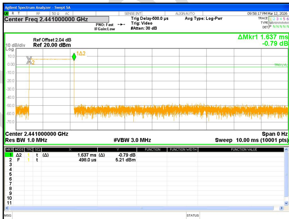
Dwell NVNT 1-DH3 2441MHz Ant1 Accumulated
