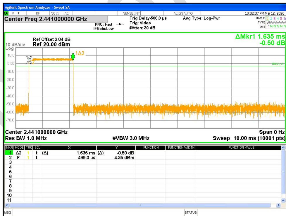
Dwell NVNT 2-DH3 2441MHz Ant1 Accumulated
