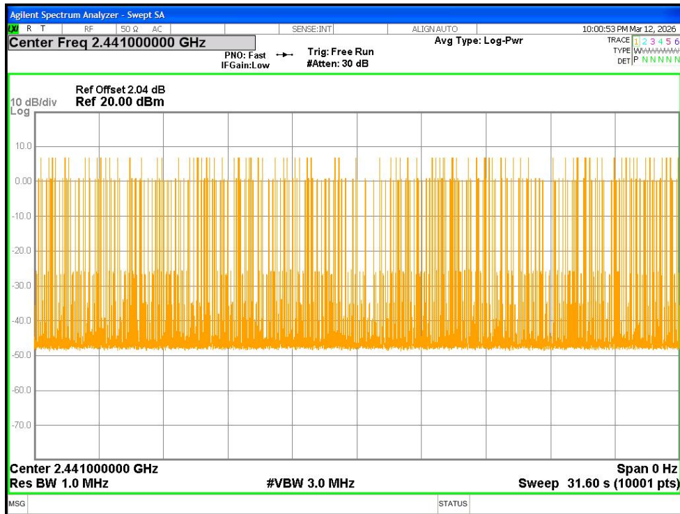
Dwell NVNT 3-DH1 2441MHz Ant1 One Burst
