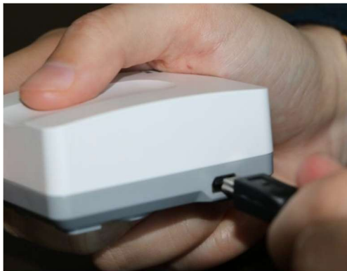
Connect the included AC power adaptor as shown. Use only the adapter that came with your Router.
