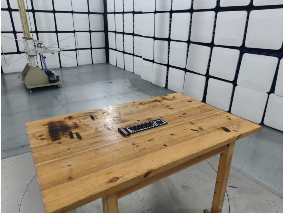
Photo of Radiation Emission Test
