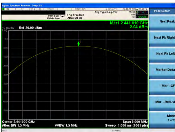
Peak output Power plot on channel 39 (1Mbps)
