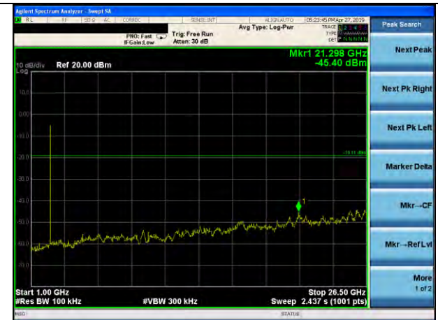
\pi/4 -DQPSK on channel 78
