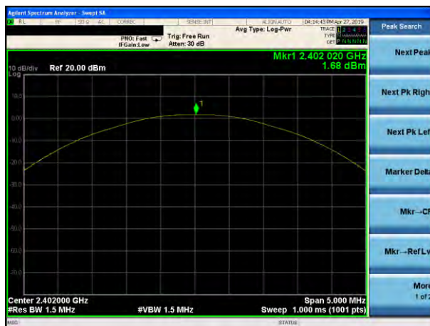
Peak output Power plot on channel 00 (2Mbps)
