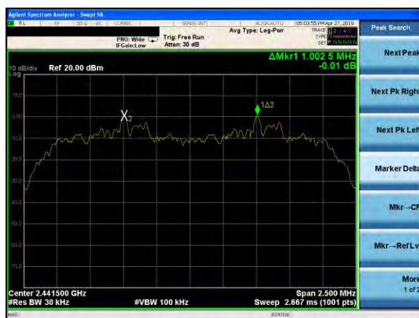
(2Mbps) Channel Separation plot on channel 39-40
