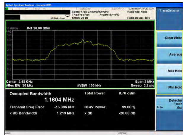
20dB Bandwidth plot on channel 78 (2Mbps)
