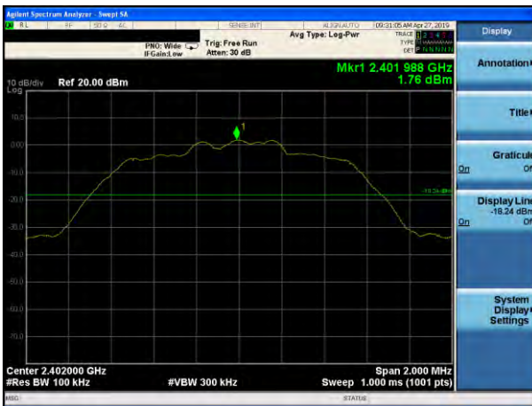
\pi/4 -DQPSK on channel 00
