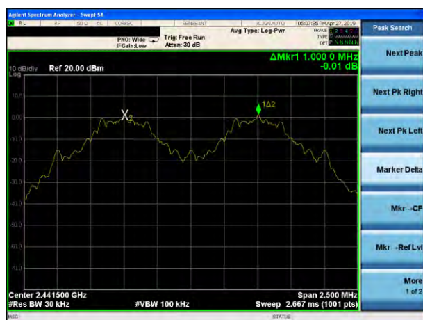
(1Mbps) Channel Separation plot on channel 39-40
