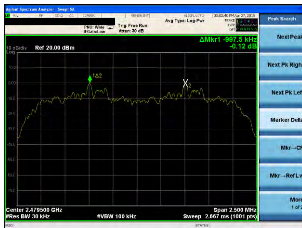
(2Mbps) Channel Separation plot on channel 77-78
