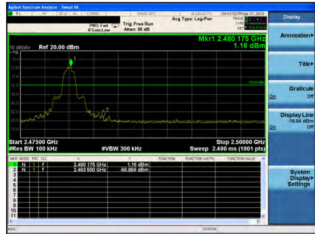
8-DPSK: Band Edge-High Channel
