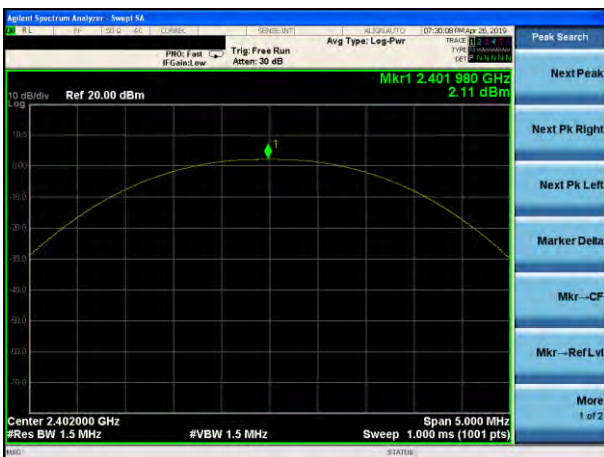
Peak output Power plot on channel 00 (1Mbps)
