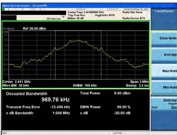
20dB Bandwidth plot on channel 78 (1Mbps)
