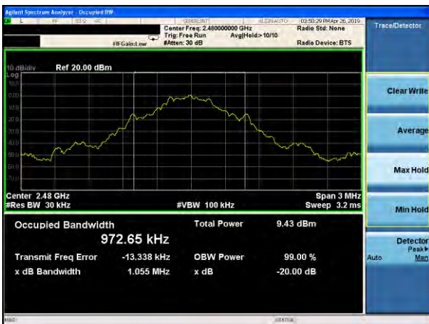
20dB Bandwidth plot on channel 78 (1Mbps)
