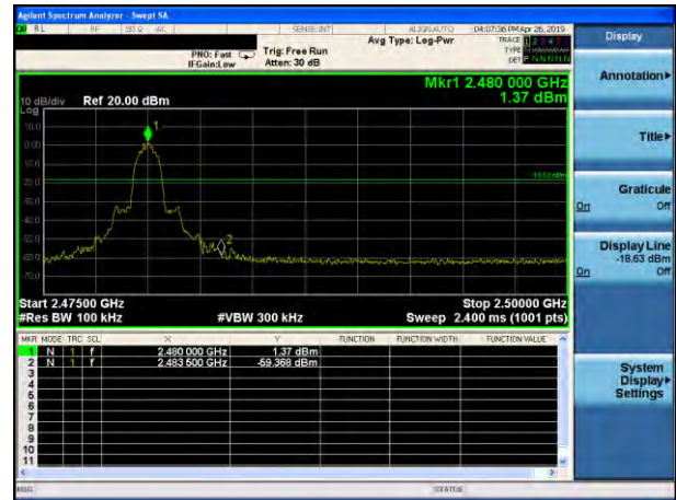
8-DPSK: Band Edge-High Channel
