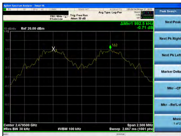
(1Mbps) Channel Separation plot on channel 77-78
