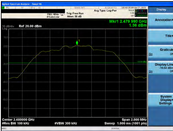
\pi/4 -DQPSK on channel 78
