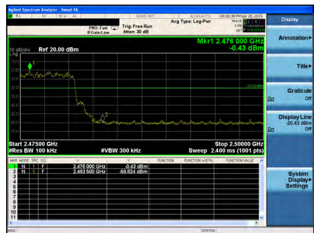
8-DPSK: Band Edge-High Channel (Hopping Mode)
