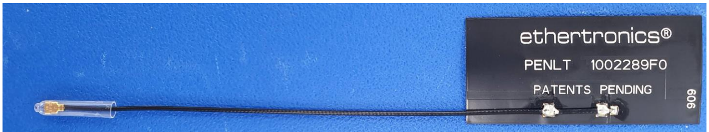
Figure 16 Top View LTE Antenna
