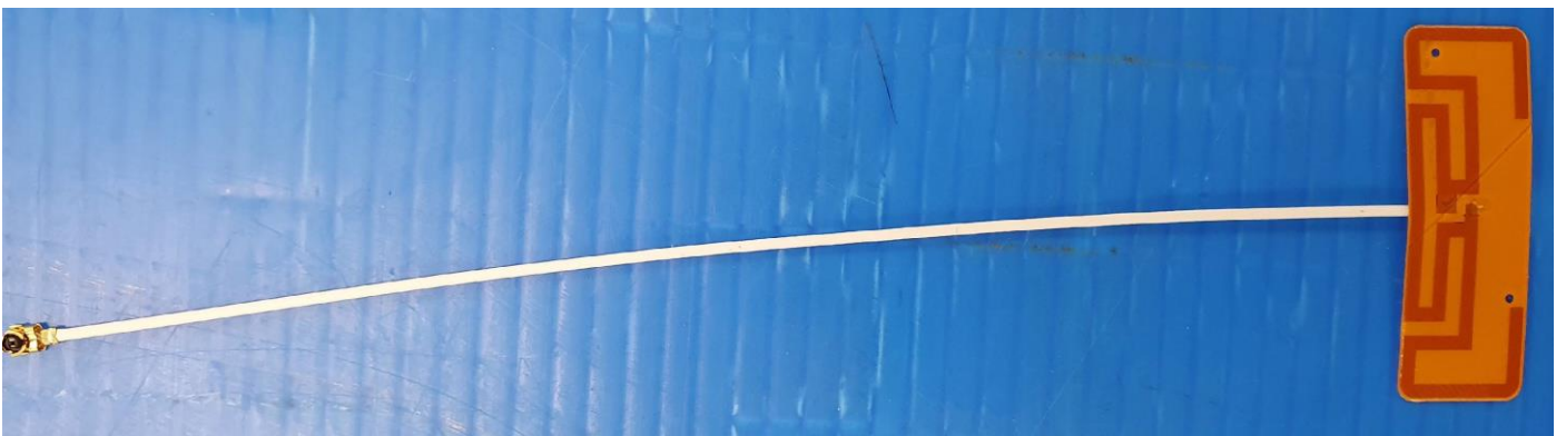
Figure 21 Bottom View GPS Antenna
