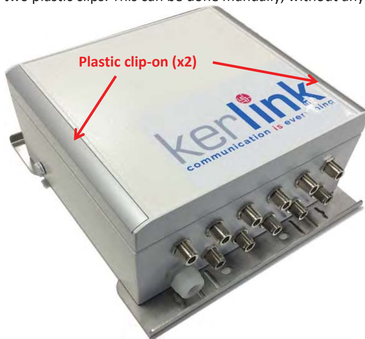
Figure 94: Wirnet iBTS – plastic clips on the lid
