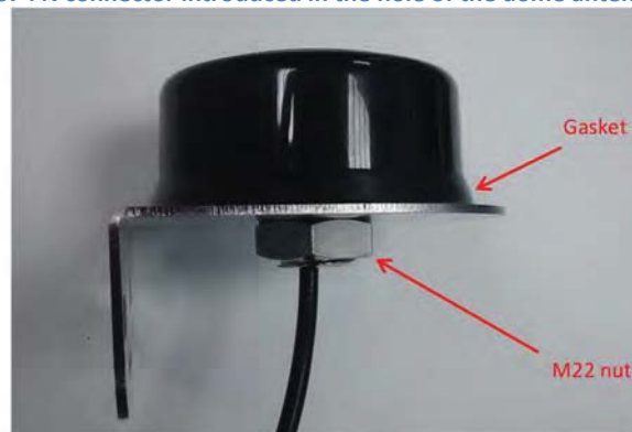
Figure 108 : Antenna installed on the dome antenna bracket
