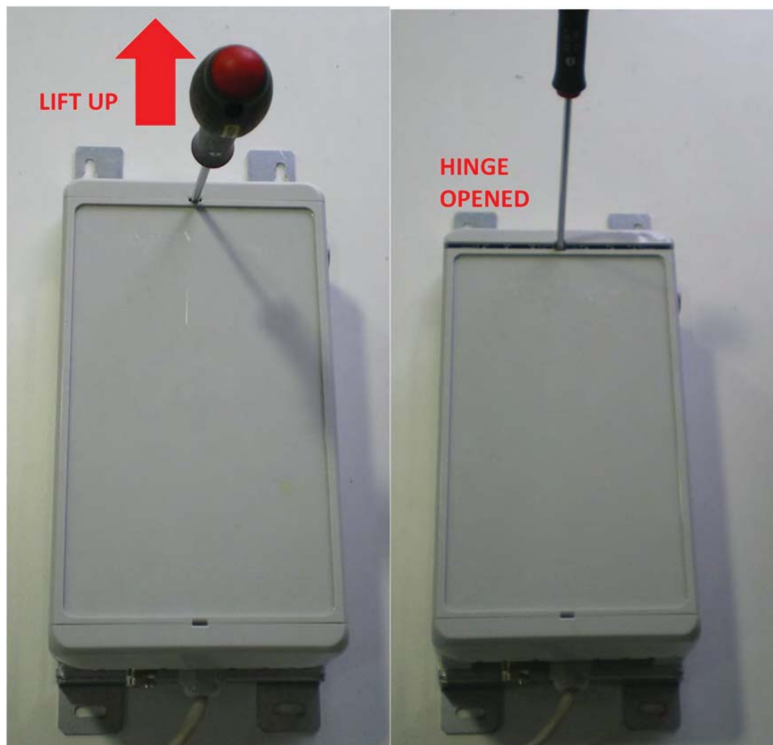
Figure 97 : Opening of the compact enclosure with screwdriver
