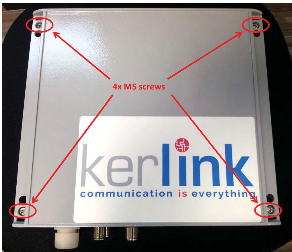
Figure 95: Wirnet iBTS – 4x M5 screws
