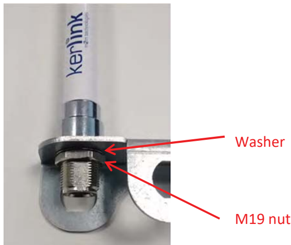
Figure 106 : LoRa antenna mounted on universal antenna bracket
