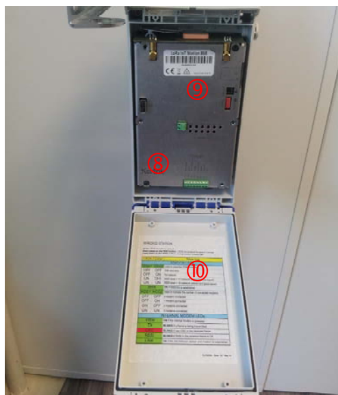
Figure 5 : LoRa IoT Station casing - internal view
