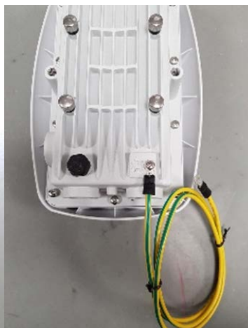
Mandatory ground connection on the Wirnet™ iStation
