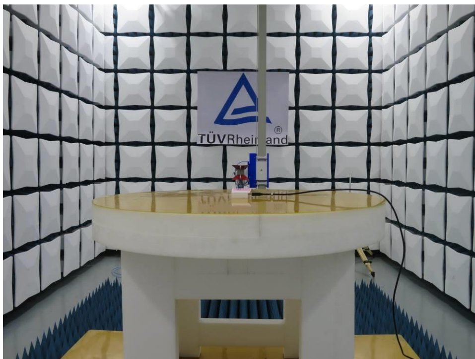
Photograph 2: Set-up for Radiated Spurious Emission, Above 1GHz
