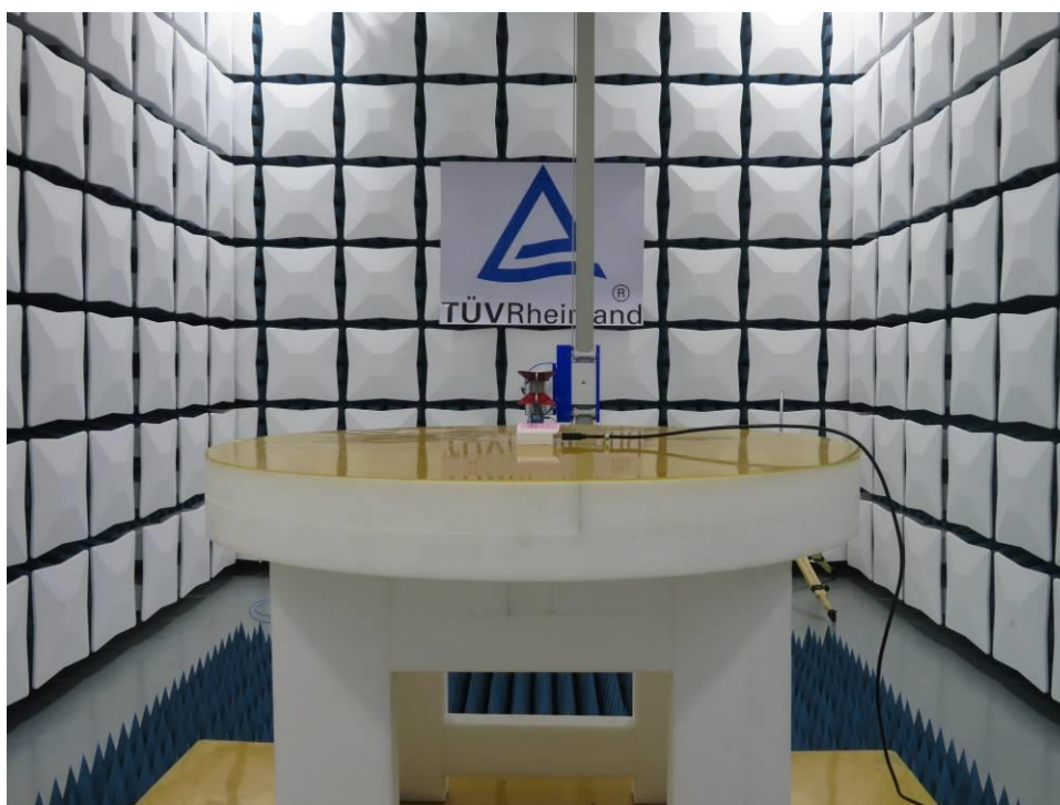
Photograph 2: Set-up for Radiated Spurious Emission, Above 1GHz
