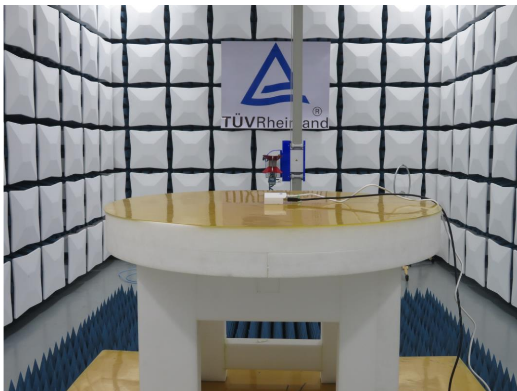
Photograph 2: Set-up for Radiated Spurious Emission, Above 1GHz
