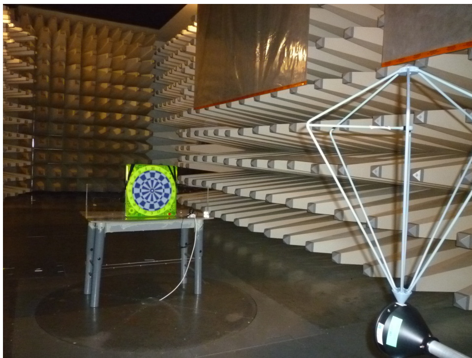
Set-up for Radiated Emission
