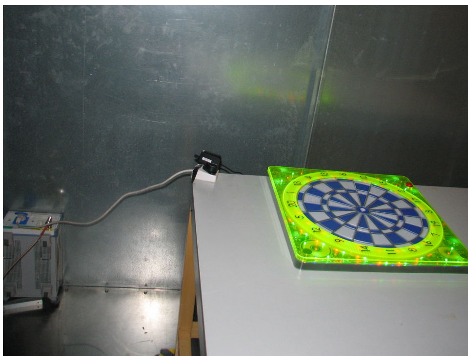
Set-up for AC Mains Conducted Emission
