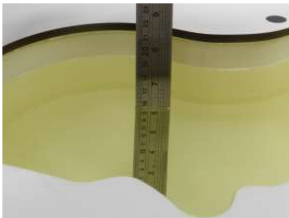
Fig 10.1 Photo of Liquid Height for Head SAR
