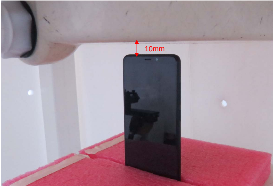
Picture 9: Top Side, the distance from handset to the bottom of the Phantom is 10mm
