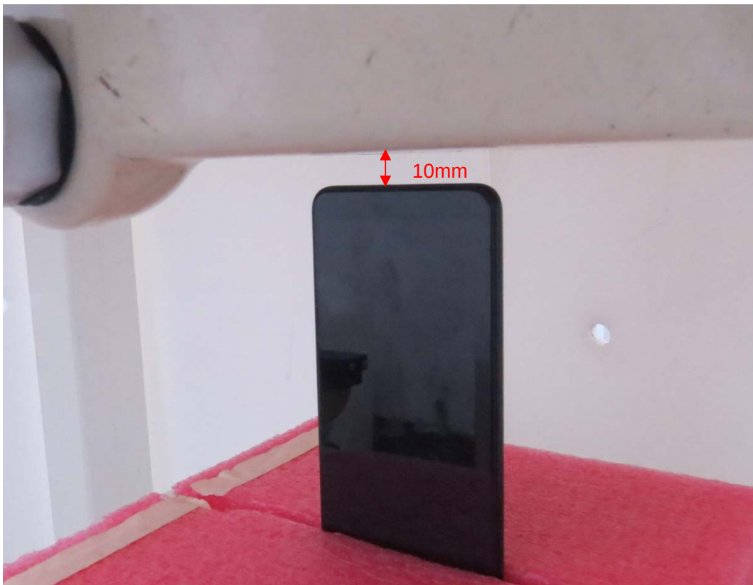
Picture 10: Bottom Side, the distance from handset to the bottom of the Phantom is 10mm
