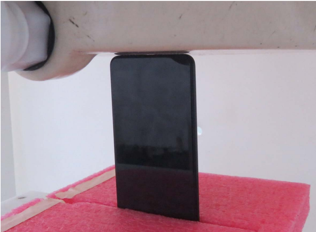
Picture 12: Bottom Side, the distance from handset to the bottom of the Phantom is 0mm
