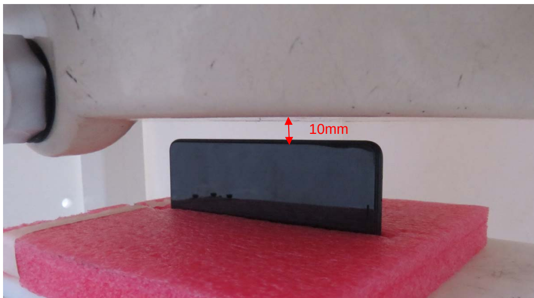
Picture 7: Left Side, the distance from handset to the bottom of the Phantom is 10mm
