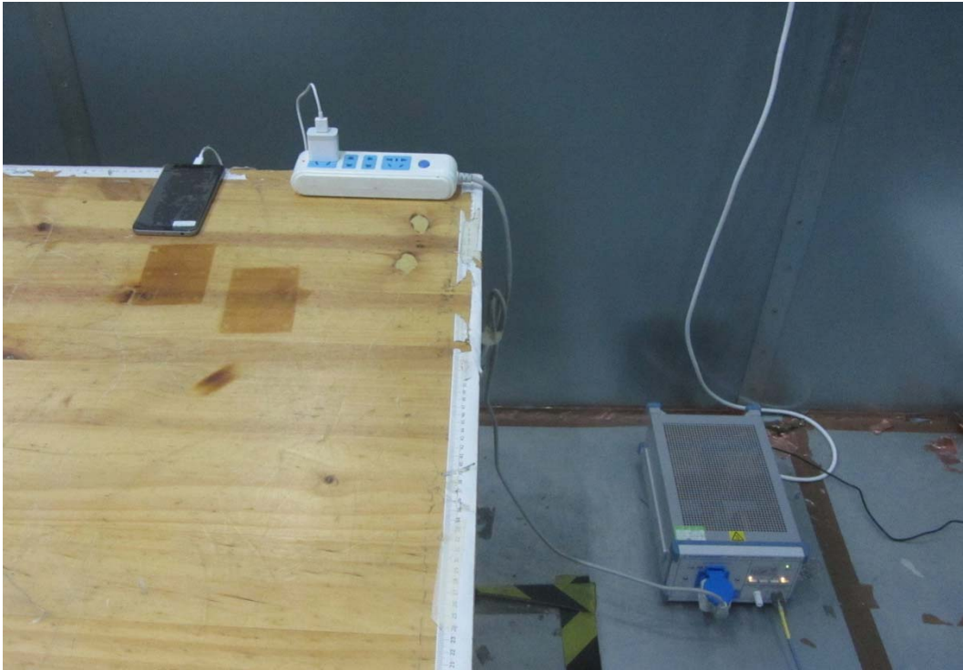
Picture 3 Conducted Emission Test Setup
