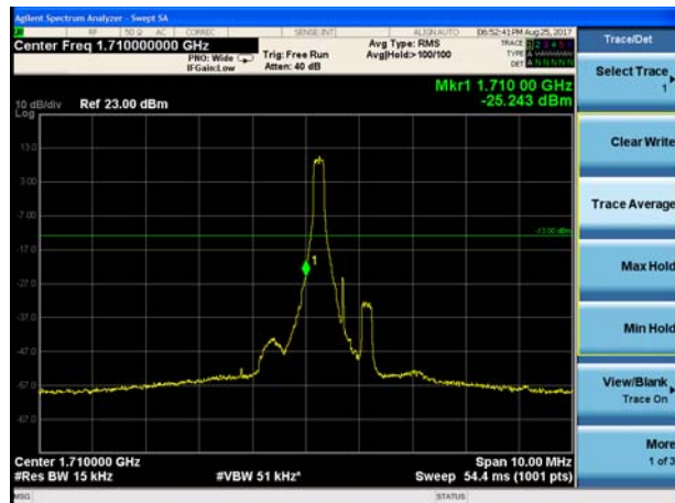
LTE Band 4 16QAM 1.4MHz CH-Low, 100%RB
