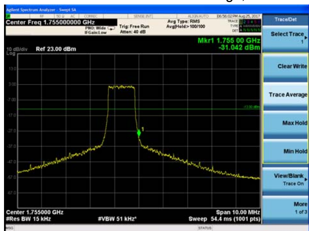
LTE Band 4 16QAM 3MHz CH-High, 1 RB
