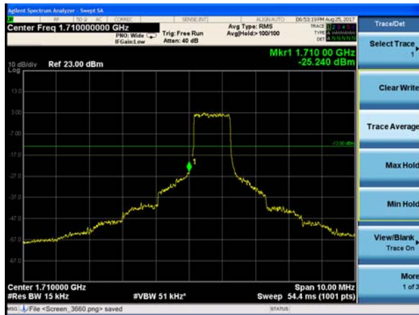
LTE Band 4 QPSK 3MHz CH-Low, 1 RB
