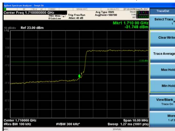
LTE Band 4 16QAM 15MHz CH-Low, 1 RB
