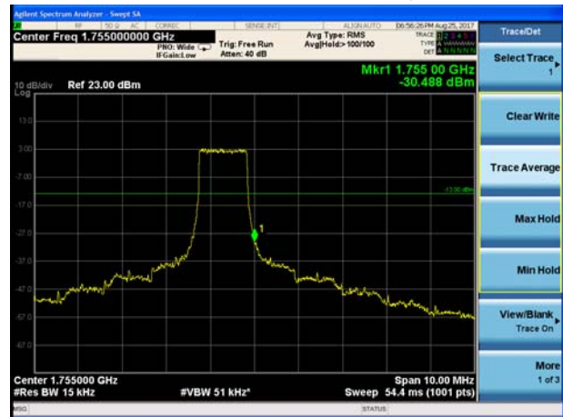
LTE Band 4 QPSK 3MHz CH-High, 1 RB
