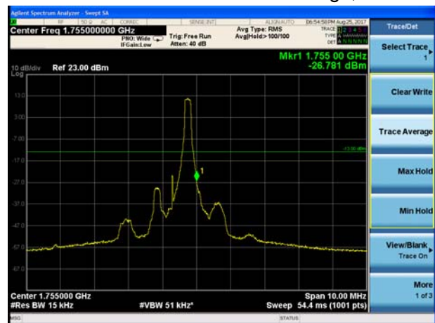
LTE Band 4 QPSK 1.4MHz CH-High, 100%RB
