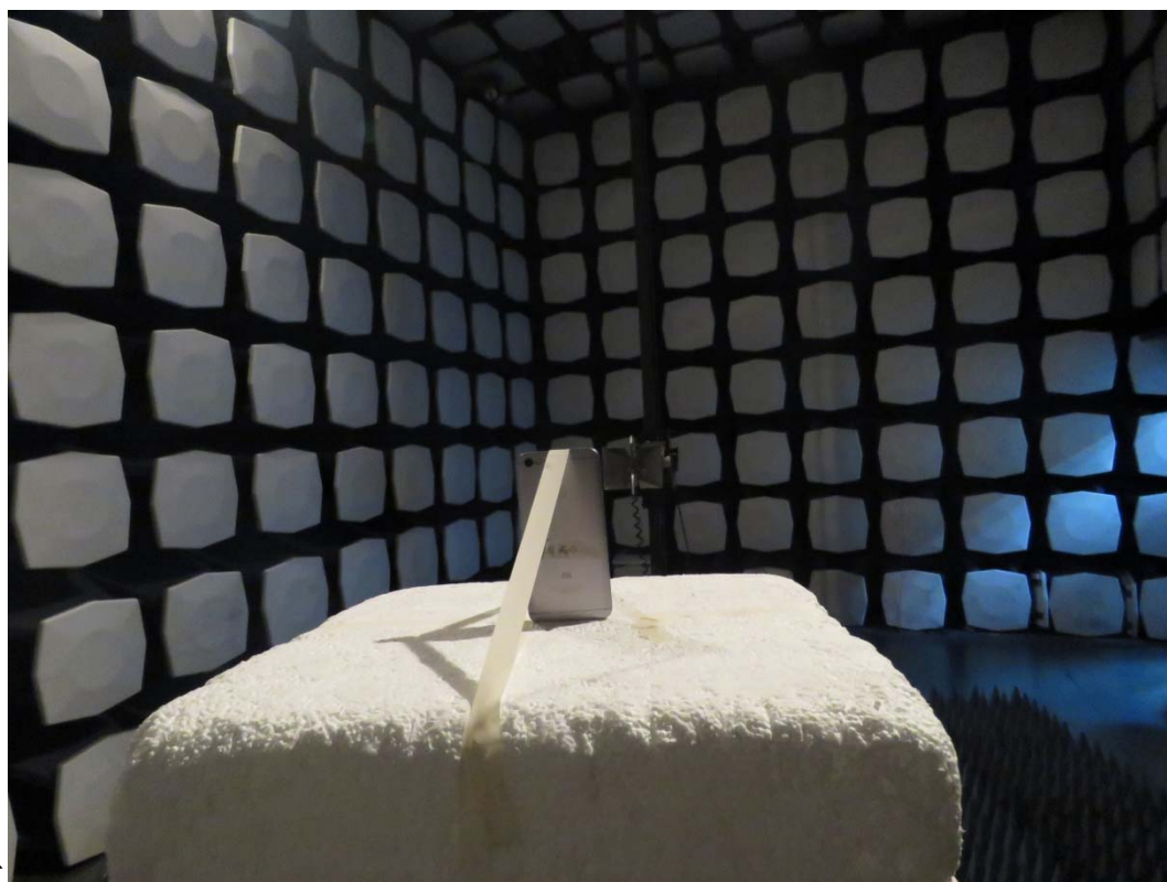
Picture 2: Radiated Spurious Emissions Test setup
