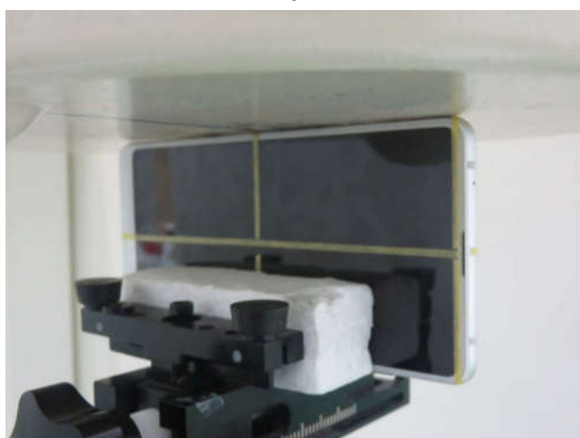
Left Side, Test Separation 0 mm
