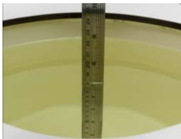
Fig 11.1.2 Photo of Liquid Height for Body SAR
