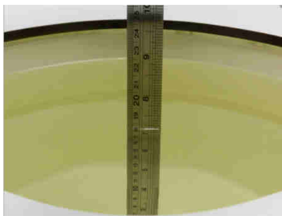
Fig 8.2 Photo of Liquid Height for Body SAR
