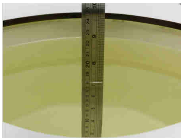
Fig 8.2 Photo of Liquid Height for Body SAR
