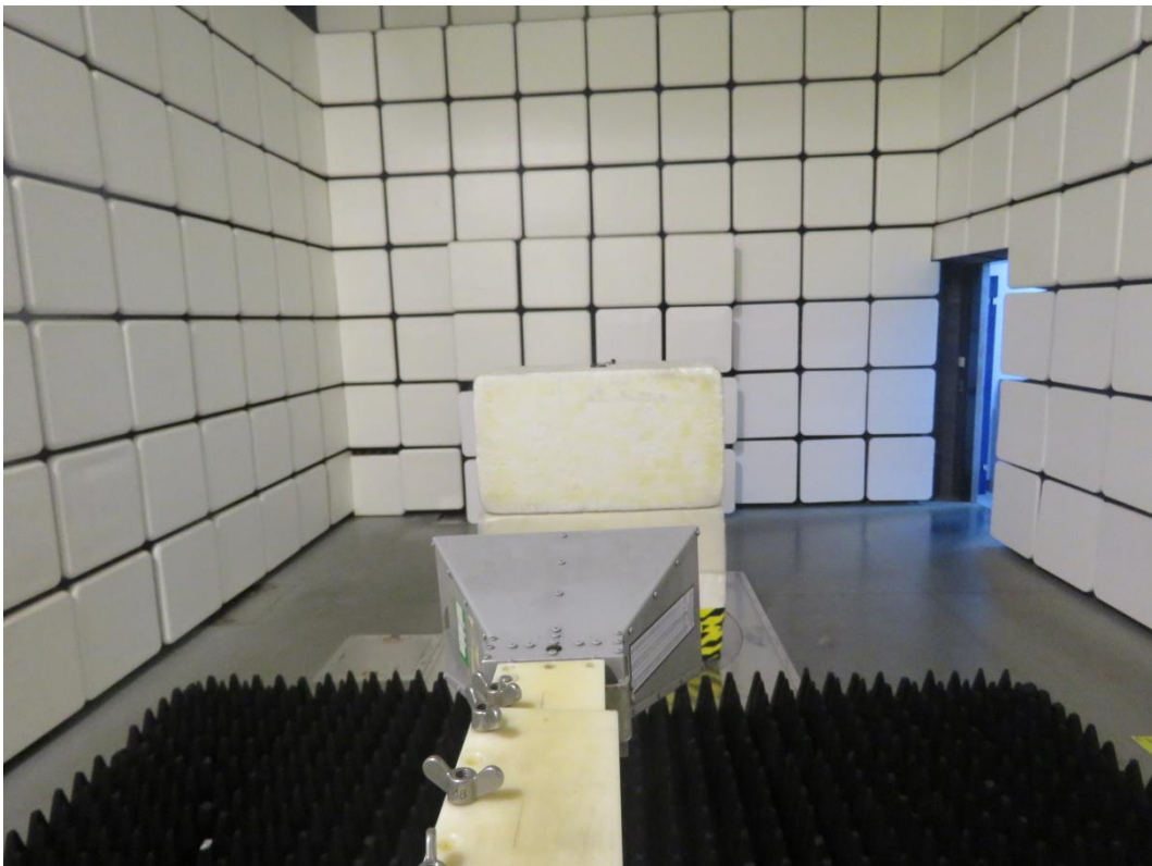
Picture 1: Radiated Spurious Emissions Test setup
