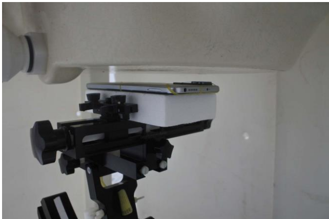
Back, Test Separation 15 mm(sensor off)
