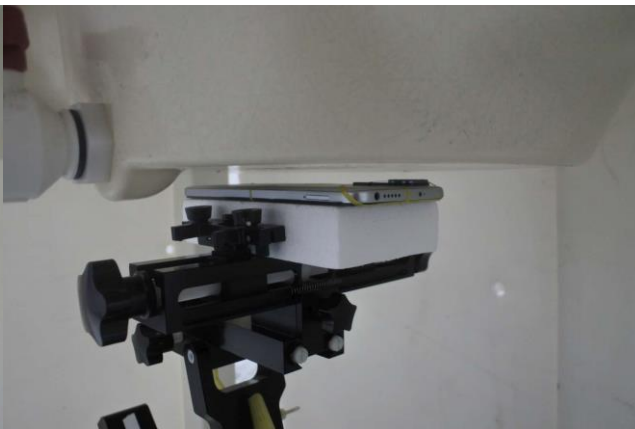
Back, Test Separation 10 mm
