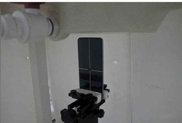
Bottom Side, Test Separation 10 mm
