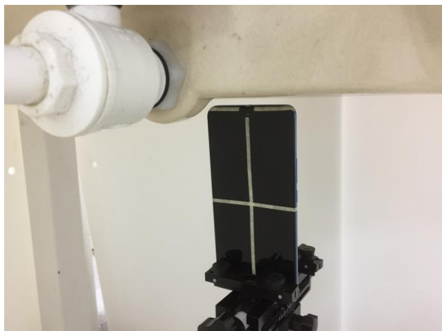
Top Side, Test Separation 5 mm
