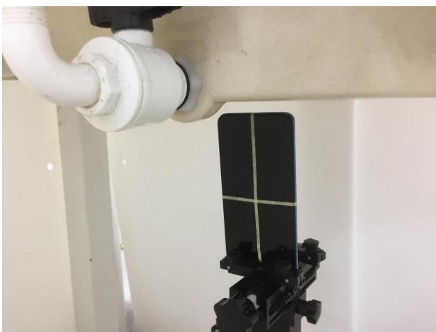
Bottom Side, Test Separation 10 mm
