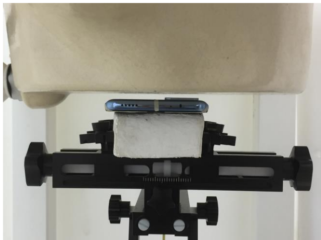
Back, Test Separation 5 mm
