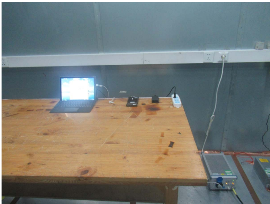
Picture 2: Conducted Emissions Test Setup
