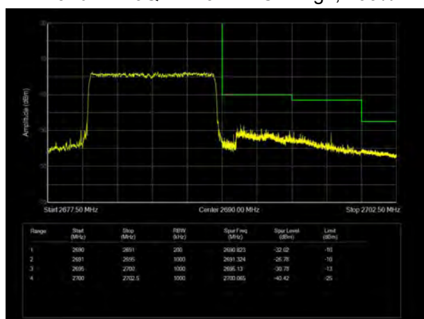
LTE Band 41 16QAM 15MHz CH-High, 1 RB
