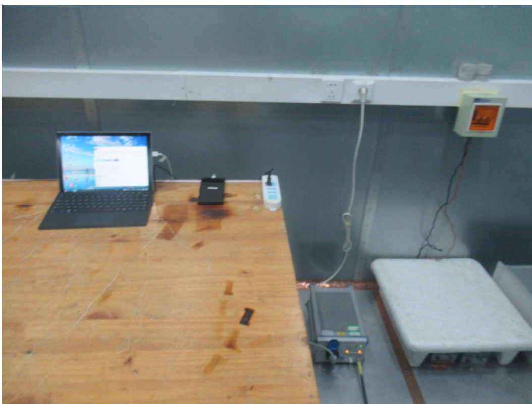
Picture 2 Conducted Emission Test Setup
