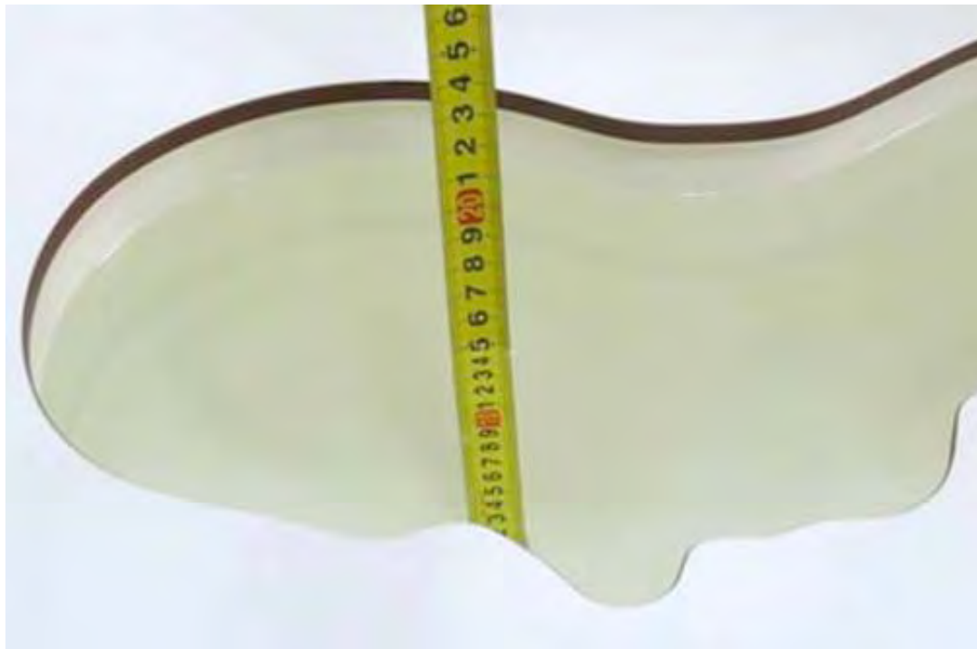
Picture 3: liquid depth in the head Phantom
