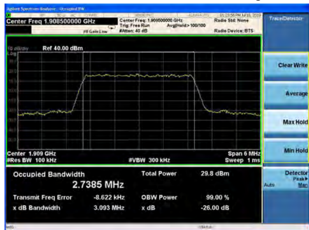
LTE Band 2 3MHz 16QAM CH-High
