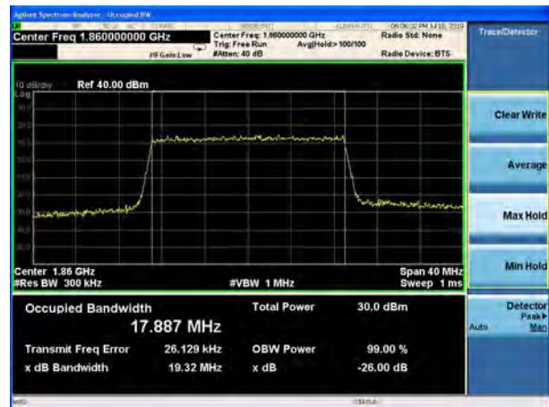
LTE Band 2 20MHz 16QAM CH-Middle
