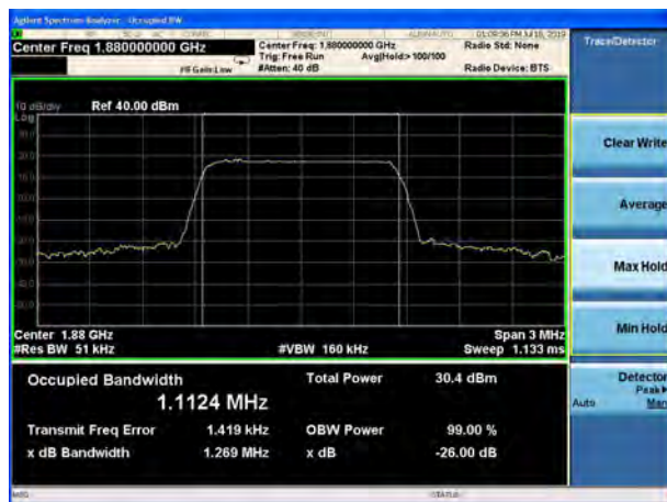
LTE Band 2 1.4MHz 16QAM CH-High
