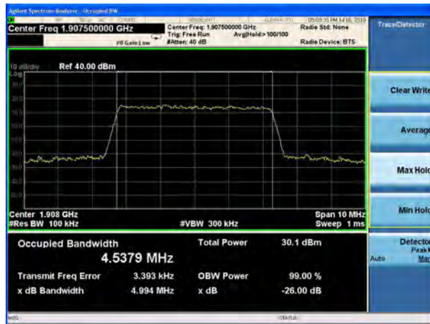
LTE Band 2 5MHz 16QAM CH-High
