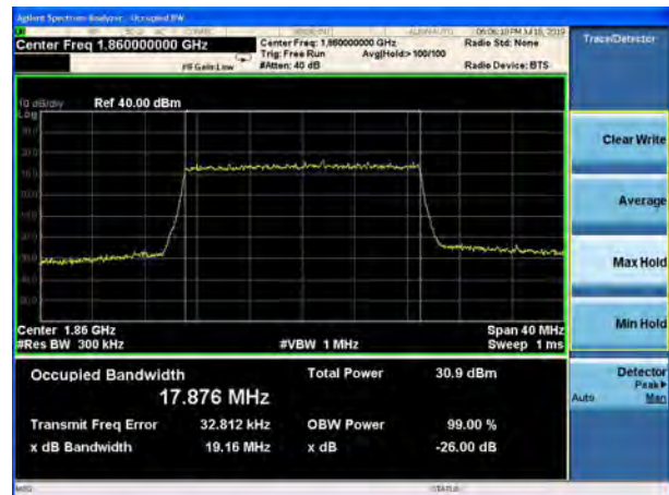
LTE Band 2 20MHz QPSK CH-Middle
