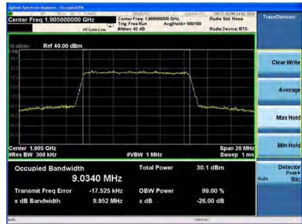
LTE Band 2 10MHz 16QAM CH-High
