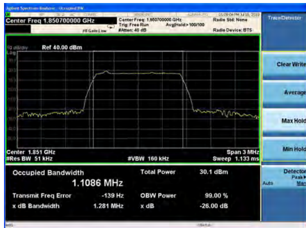
LTE Band 2 1.4MHz 16QAM CH-Middle
