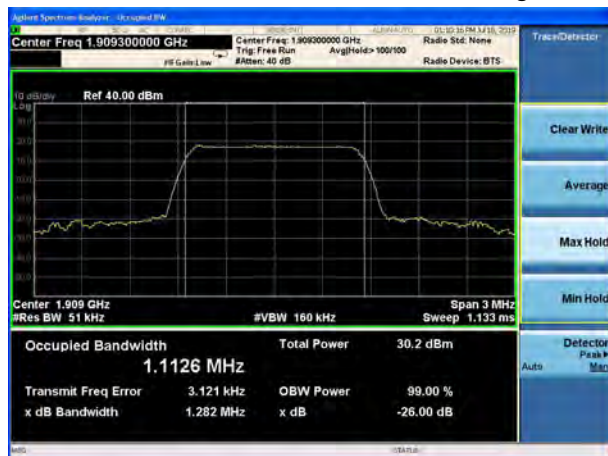
LTE Band 2 1.4MHz 16QAM CH-High
