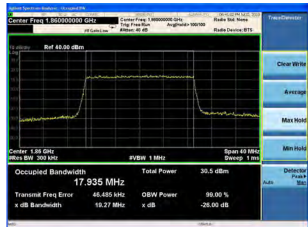
LTE Band 2 20MHz 64QAM CH-Middle
