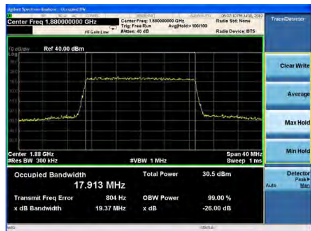
LTE Band 2 20MHz 16QAM CH-High
