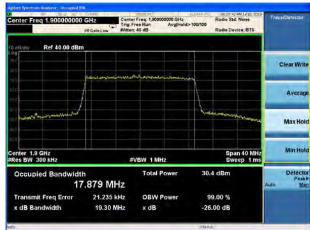
LTE Band 2 20MHz 16QAM CH-High
