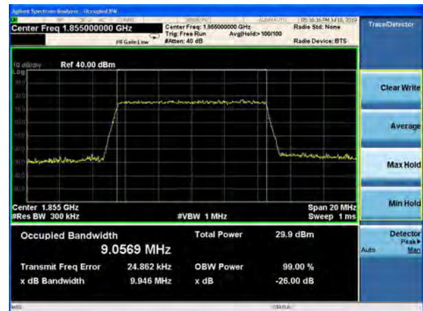
LTE Band 2 10MHz 16QAM CH-Middle
