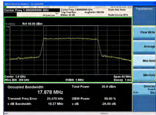
LTE Band 2 20MHz 64QAM CH-High
