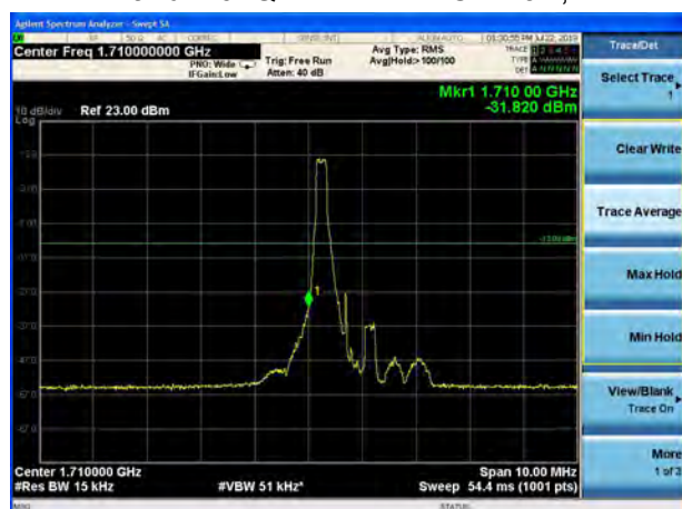
LTE Band 4 64QAM 1.4MHz CH-Low, 100%RB
