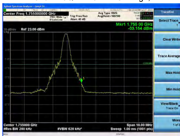
LTE Band 4 16QAM 20MHz CH-High, 1 RB
