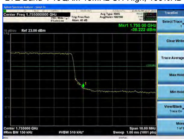
LTE Band 4 16QAM 20MHz CH-High, 1 RB
