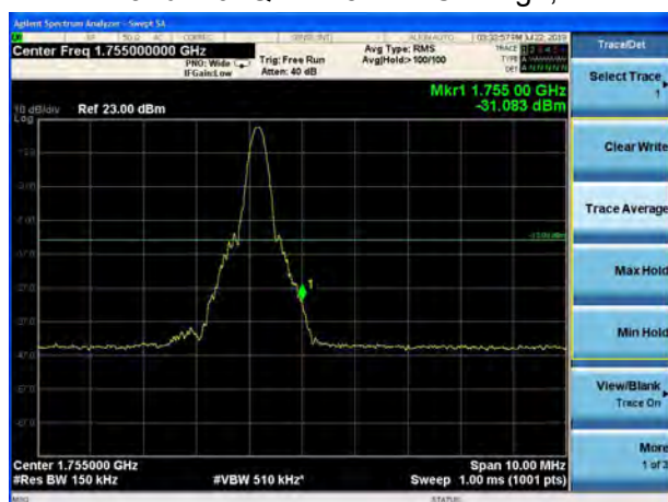
LTE Band 4 64QAM 15MHz CH-High, 100%RB
