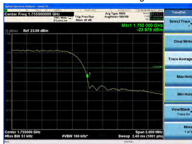
LTE Band 4 QPSK 1.4MHz CH-High, 1 RB
