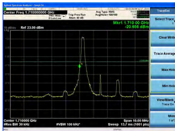
LTE Band 4 16QAM 3MHz CH-Low, 100%RB
