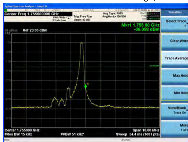
LTE Band 4 QPSK 1.4MHz CH-High, 100%RB
