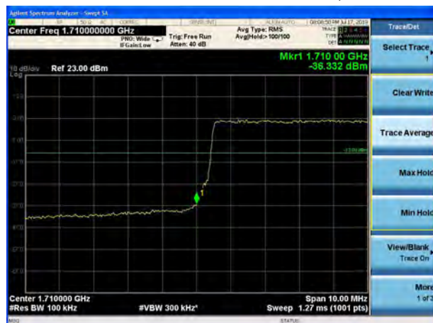
LTE Band 4 16QAM 10MHz CH-Low, 100%RB
