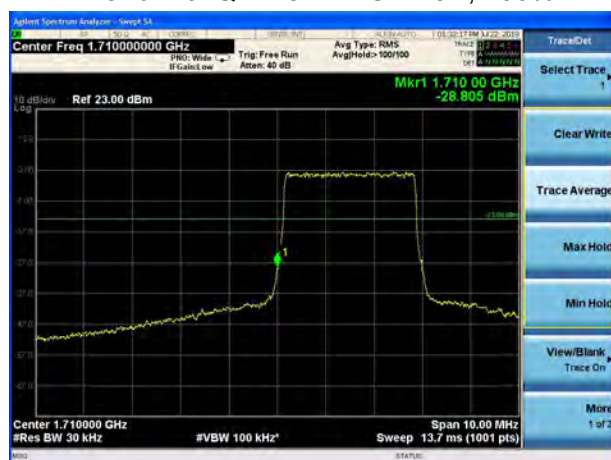
LTE Band 4 64QAM 5MHz CH-Low, 1 RB
