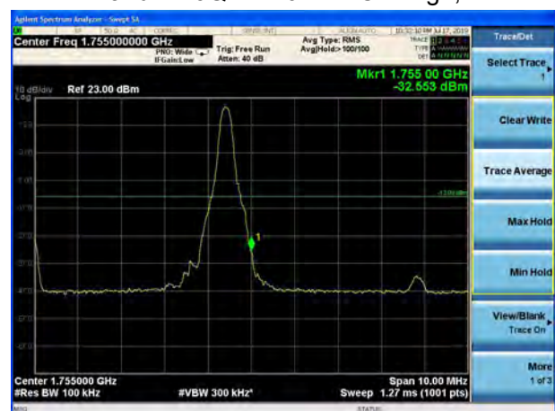
LTE Band 4 16QAM 10MHz CH-High, 100%RB
