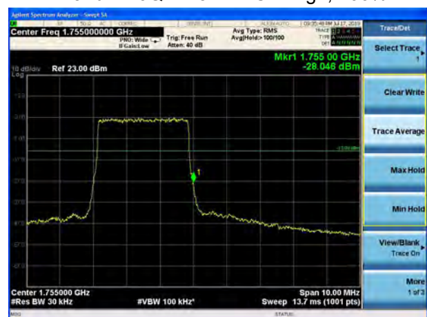
LTE Band 4 16QAM 5MHz CH-High, 1 RB
