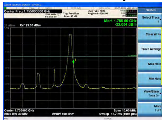
LTE Band 4 16QAM 3MHz CH-High, 100%RB
