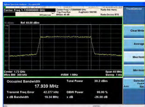
LTE Band 4 64QAM 20MHz CH-Middle
