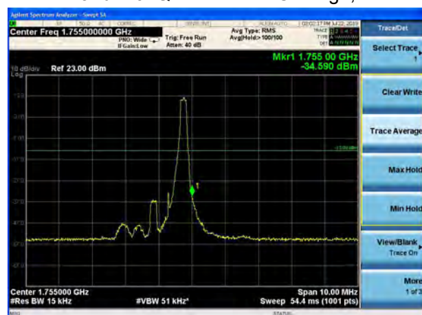
LTE Band 4 64QAM 1.4MHz CH-High, 100%RB
