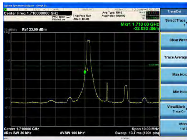
LTE Band 4 64QAM 3MHz CH-Low, 100%RB
