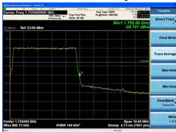
LTE Band 4 QPSK 10MHz CH-High, 1 RB
