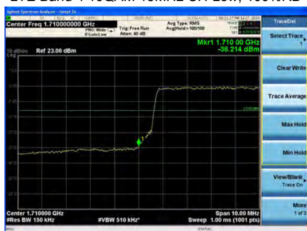
LTE Band 4 16QAM 20MHz CH-Low, 1 RB
