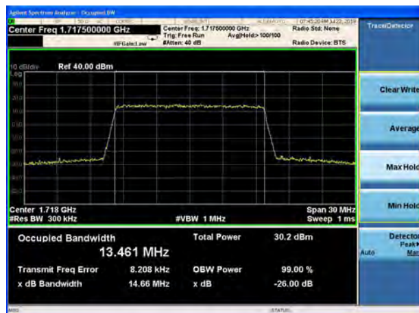
LTE Band 4 64QAM 15MHz CH-Middle
