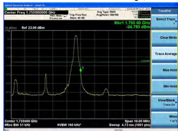
LTE Band 4 16QAM 5MHz CH-High, 1 RB
