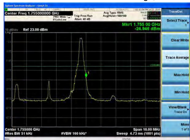
LTE Band 4 64QAM 5MHz CH-High, 1 RB
