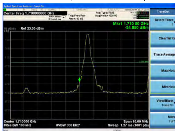
LTE Band 4 16QAM 10MHz CH-Low, 100%RB
