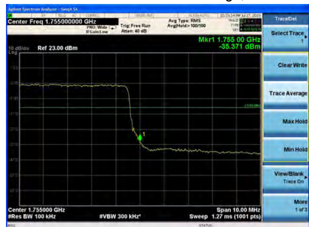
LTE Band 4 16QAM 10MHz CH-High, 100%RB
