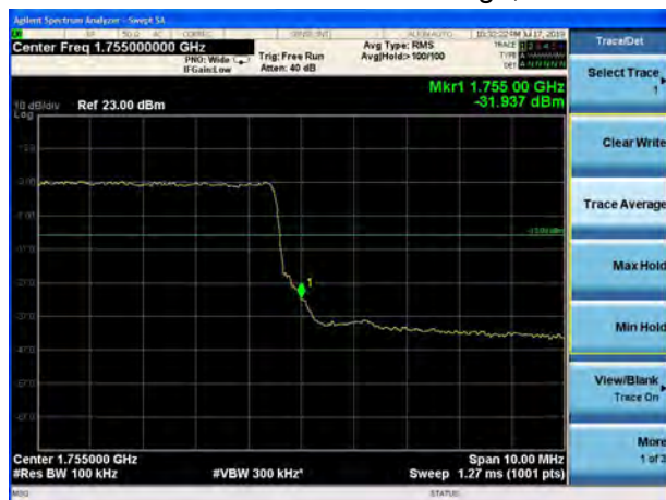
LTE Band 4 QPSK 10MHz CH-High, 100%RB
