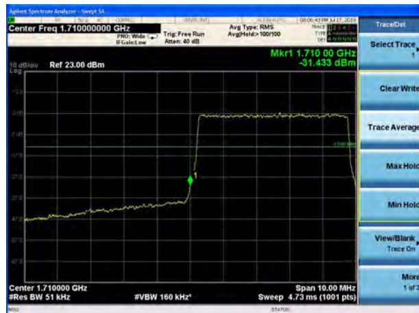
LTE Band 4 16QAM 10MHz CH-Low, 1 RB
