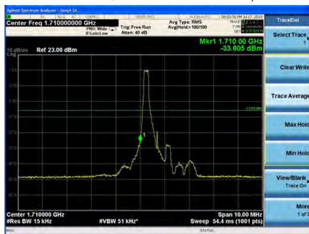
LTE Band 4 QPSK 1.4MHz CH-Low, 100%RB
