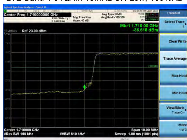
LTE Band 4 64QAM 20MHz CH-Low, 1 RB
