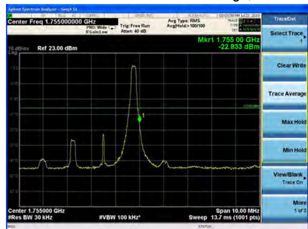
LTE Band 4 64QAM 3MHz CH-High, 100%RB
