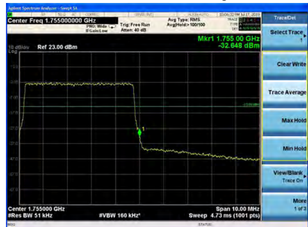
LTE Band 4 16QAM 10MHz CH-High, 1 RB
