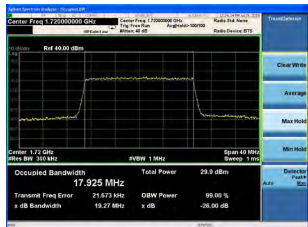
LTE Band 4 16QAM 20MHz CH-Middle
