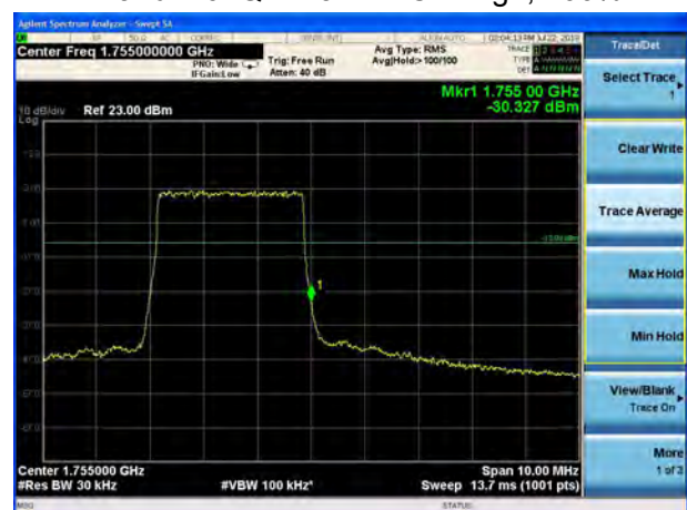
LTE Band 4 64QAM 5MHz CH-High, 1 RB
