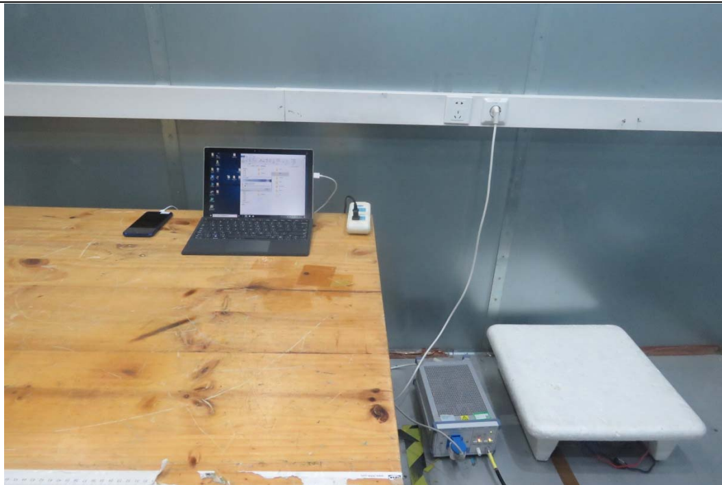
Picture 2 Conducted Emission Test Setup
