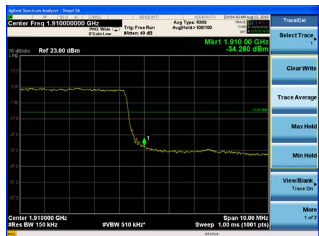
LTE Band 2 20MHz 64QAM 1RB CH-High
