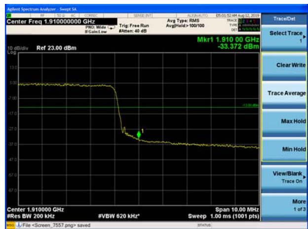
LTE Band 2 1.4MHz 16QAM 1RB CH-High
