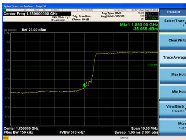
LTE Band 2 20MHz 16QAM 1RB CH-Low
