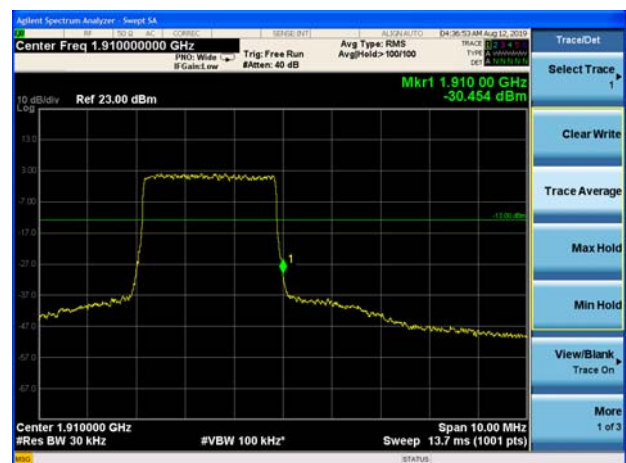
LTE Band 2 5MHz 64QAM 1RB CH-High
