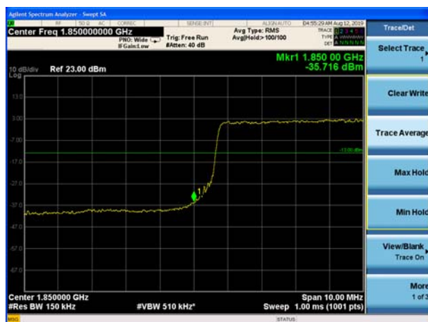
LTE Band 2 20MHz 64QAM 1RB CH-Low
