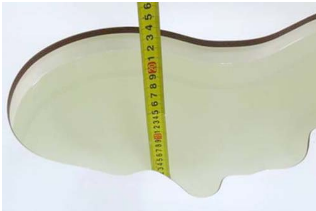
Picture 3: liquid depth in the head Phantom
