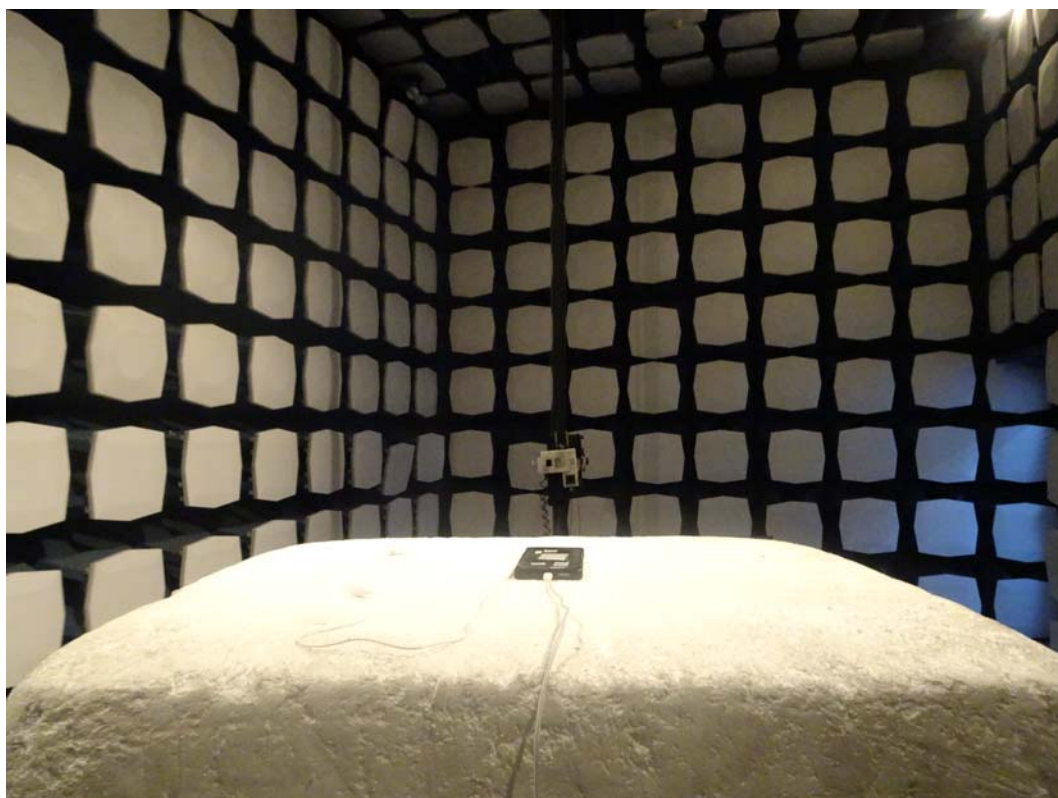
Picture 1: Radiated Spurious Emissions Test setup
