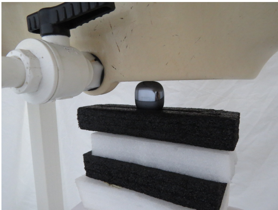
Picture 5: Top Edge, the distance from EUT to the bottom of the Phantom is 0mm
