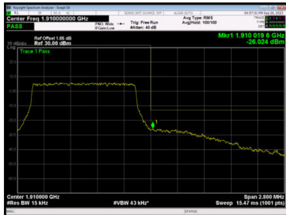
LTE Band 2 3MHz QPSK 1RB CH-High
