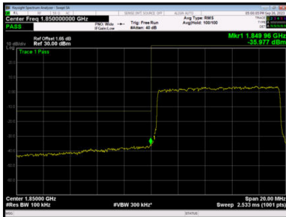
LTE Band 2 15MHz 64QAM 1RB CH-Low
