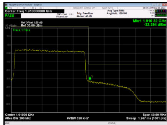
LTE Band 2 20MHz 64QAM 100%RB CH-High
