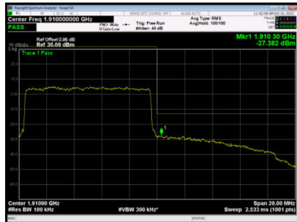
LTE Band 2 15MHz QPSK 1RB CH-High
