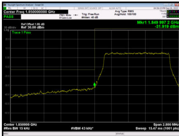
LTE Band 2 3MHz QPSK 1RB CH-Low
