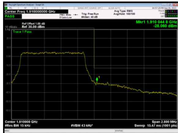
LTE Band 2 3MHz 64QAM 1RB CH-High
