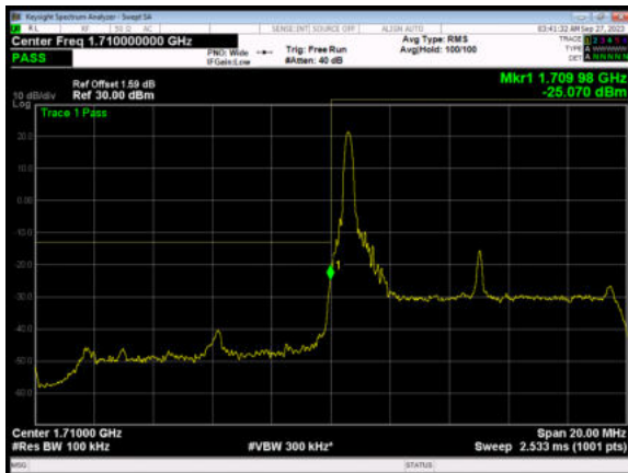
LTE Band 66 64QAM 10MHz CH-Low, 100%RB
