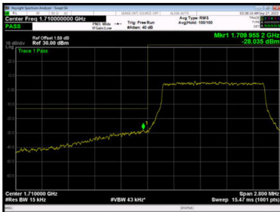
LTE Band 66 64QAM 3MHz CH-Low, 1 RB
