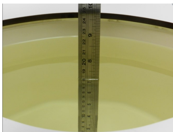
Fig 11.1.2 Photo of Liquid Height for Body SAR
