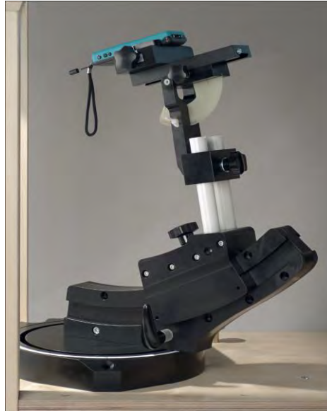
F-2. Device Holder for Transmitters
