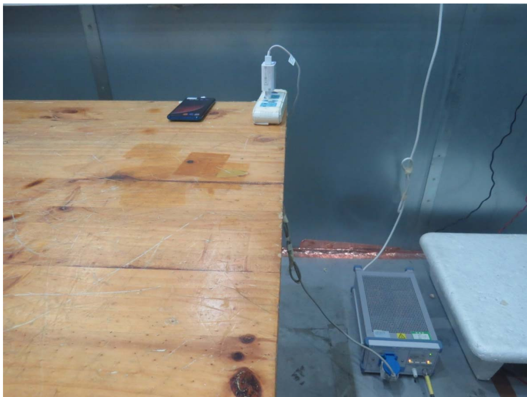
Picture 2 Conducted Emission Test Setup
