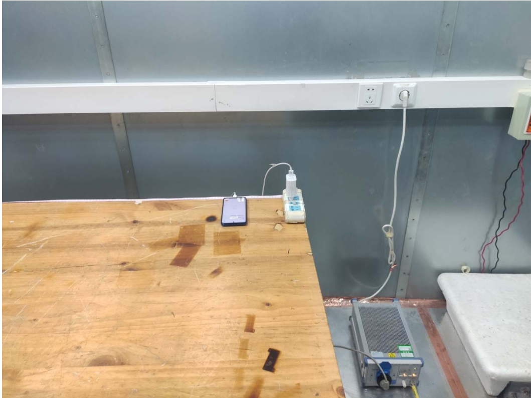
Picture 2 Conducted Emission Test Setup
