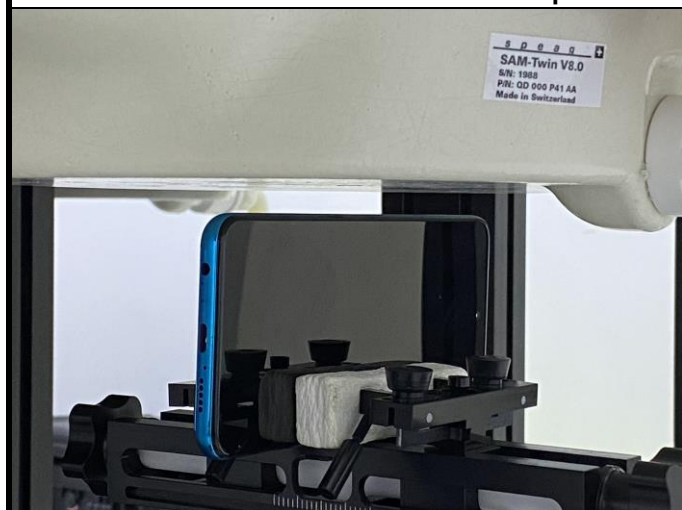
Left Side of EUT with 1.0 cm Gap
