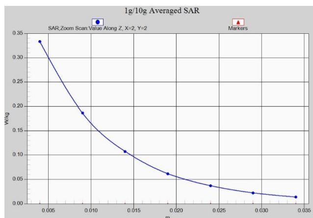
Fig. 1-4 Z-Scan at power reference point (PCS1900)
