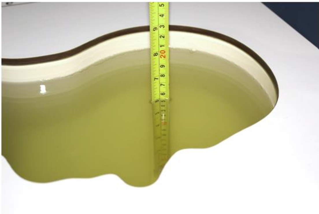
Picture 7-5 Liquid depth in the Head Phantom (2600 MHz)
