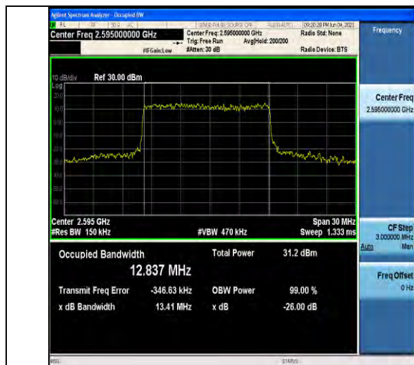
NTNV-N38-30kHz-15MHz-DFT-256QAM- Mid-Outer Full-----PASS
