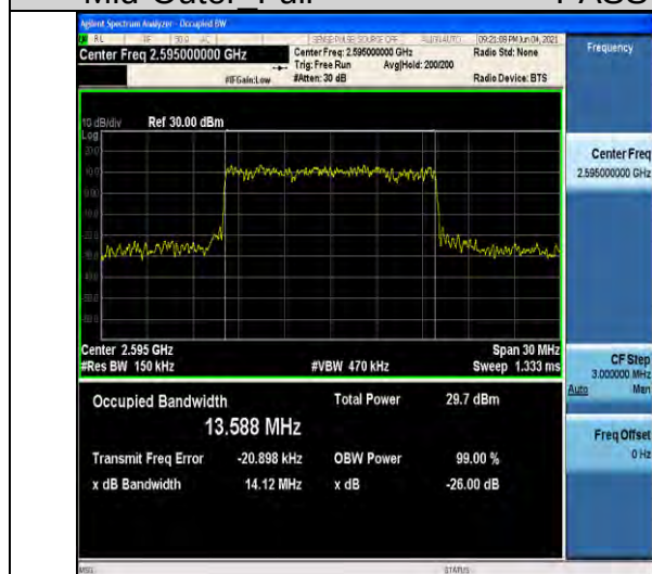
NTNV-N38-30kHz-15MHz-CP-16QAM-Mid- Outer Full-----PASS
