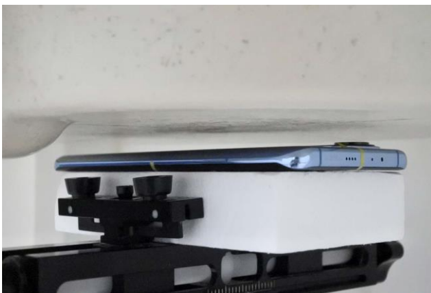
Back, Test Separation 10 mm
