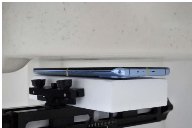
Front, Test Separation 10 mm
