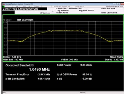
BLE (1M) Carrier frequency (MHz): 2480
