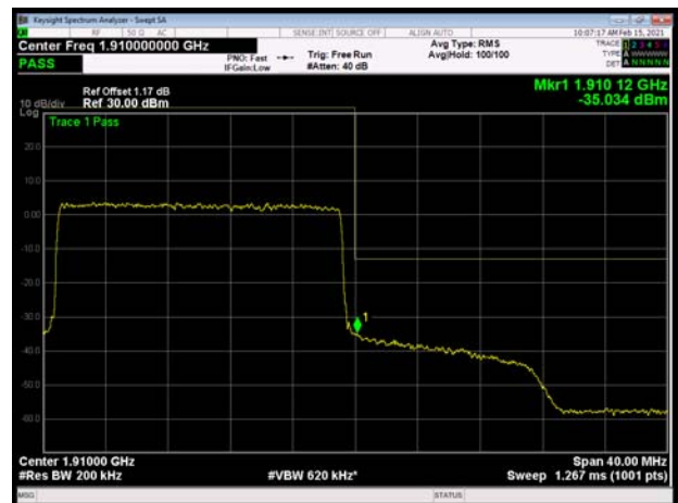
LTE Band 2 20MHz 64QAM 100%RB CH-High
