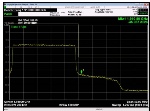
LTE Band 2 20MHz 16QAM 100%RB CH-High
