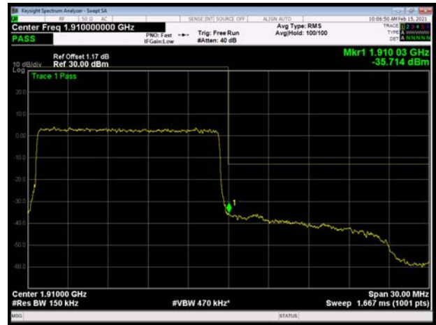
LTE Band 2 20MHz 64QAM 1RB CH-High
