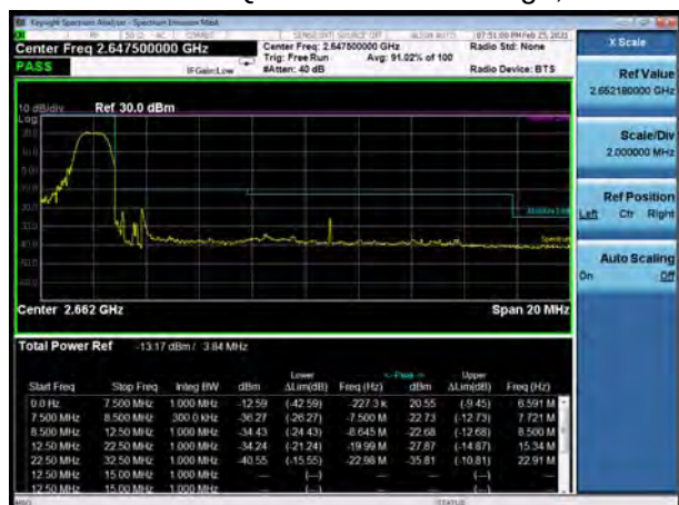
LTE Band 41 QPSK 15MHz CH-High, 1 RB
