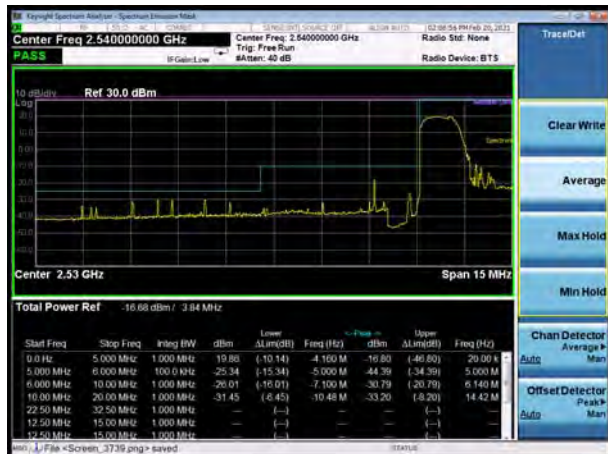
LTE Band 41 64QAM 10MHz CH-Low, 100%RB
