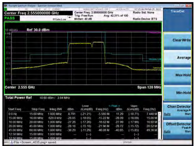
CA_7C 64QAM 20MHz+10MHz CH-High, 100%RB
