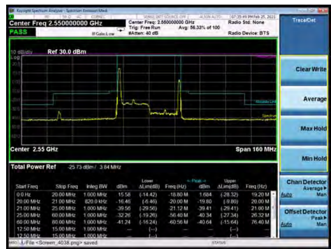
CA_7C 64QAM 20MHz+20MHz CH-High, 1 RB
