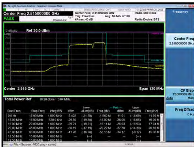
CA_7C 64QAM 20MHz+10MHz CH-Low, 100%RB
