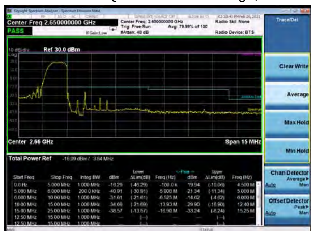
LTE Band 41 QPSK 10MHz CH-High, 100%RB
