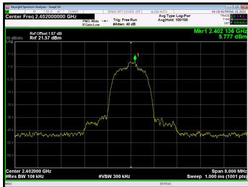
BT 2DH5 CH0, Carrier frequency (MHz): 2402
